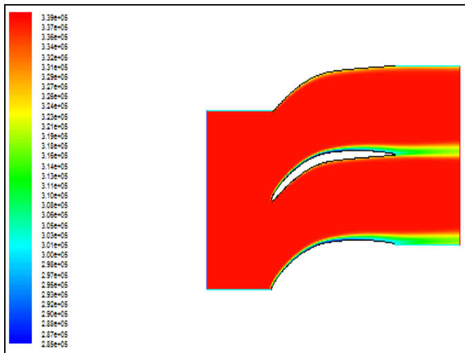
Fig. 8. Total pressure contours
